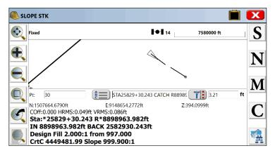
Note that because the GPS reads continuously and models the ground surface, the program calculates immediately where the catch point (the circle with the X) is located. You simply walk right to it. If the ground goes uphill or downhill as you approach the point, then the X will move closer or move away, until you are right on it. As you get closer to the point (within the stake tolerance distance) the program will present a bullseye screen.
