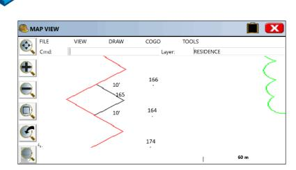
For L-shaped figures, offsets are also projected through to the other side, so that the offset for point 174 appears across the building, for purposes of pulling a stringline.
