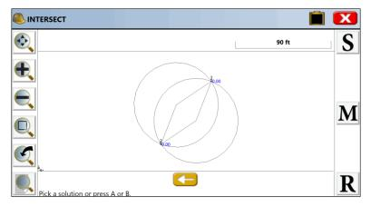
Select **OK**, and the map screen will display showing circles radiating from the first and second selected base points. Lines leading from both base points to the two possible intersections of the circles are also shown.
