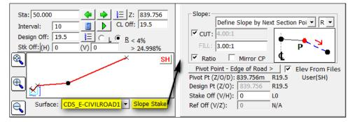
Slope Staking takes you to a "parameter" dialog where you set the Pivot Point type (here it is "User Selection") and how the next slope is defined. By selecting "Define Slope by Next Section Point", the program detects that point is in cut, so calculates the cut upslope at 4:1 (matching the >25% at left) and ghosts the value so it cannot be changed. You can also change the selection type to "User Defined" and enter any cut upslope ratio you prefer. Then click the Green Check (OK) to continue:
