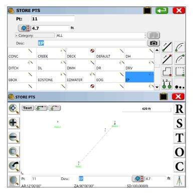
Unless the rod **hgt/description** prompt is enabled, the **Store Points** screen is designed to "quick-store" points, where the user is expected to enter, ahead of time, the correct description and rod heights in the edit boxes shown at the bottom of the dialog.
