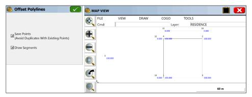
For L-shaped buildings or figures with angles, an additional interior offset point is calculated at the intersect of the parallel offset lines based on the entered offset distance, such as 10 (see point 165 below--the lines to 165 are drawn only to illustrate the 10' offset):
