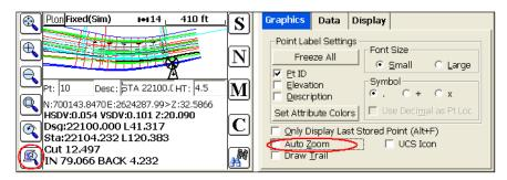
When "Auto Zoom" is clicked on, the program zooms closely as the target is approached, leading to the bullseye (which appears whenever the target is within the Stakeout Tolerance set within Equip Menu, Tolerances.
