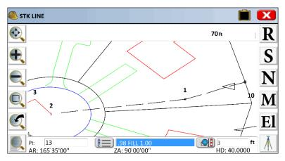
**Total Stations/GPS, Perpendicular to Line**: When configured for the Perpendicular to Line method, the program will show the direction and distance to move to find the nearest point on the line to the measured point. The instruction received (In/Out versus North/South or Azimuth/Distance) will depend on the setting within Configure Reading.
