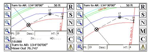
For robotic total stations in tracking mode and for GPS, the "None" setting in ViewPt, Maximized Map shows only the target and the lower line at right. In this case, the "Navigate Data" setting is beneficial. This adds an extra instruction line. Shown below is Stakeout with Navigate Data set for Maximized Map within ViewPt, running a robotic total station in tracking mode.
