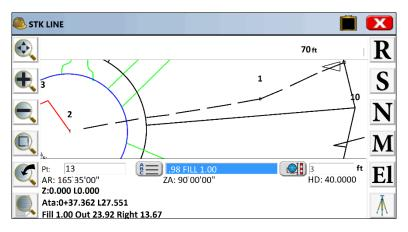
The "Turn to AR" advice at the top of the screen refers to the angle to turn to intersect the defined line at 90 degrees from the instrument location. For GPS, the Point-On-Line screen instructions are similar.
