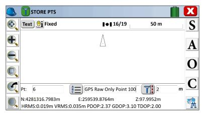
Storing a point will automatically set the user to the Average screen where the Readings Per Point will be initiated and averaged.
