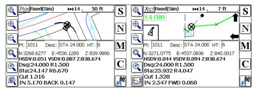
The process can be repeated for the cul-de-sac. Here we will stake out both the stone subgrade outside point and then we will slope stake the catch at a station approximately 1/4 of the distance around the cul-de-sac:
