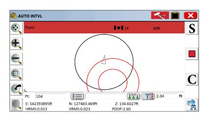
As soon as the receiver is level for the specified length of time, a point will be stored. If you selected the Audio option in Equip – GPS Rover, an audible alert will sound.
