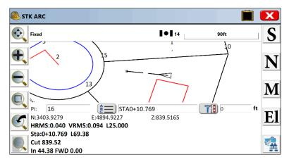
The above example might be useful for setting stakes at a 25' building setback from the right-of-way line. For GPS, information is provided "real-time". As you move, you see the instructions to contact the nearest point on the arc (or offset to the arc). For total stations, you are first instructed to measure to the nearest point on the arc (or arc offset) from the instrument setup. Then after you take any shot, the instruction refers to that measurement.
