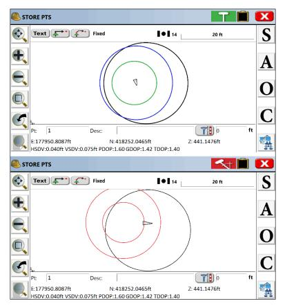
Users who wish to stay within level tolerance but do not like the appearance of the digital level can simply turn off View GNSS Level in the configure screen. As long as the IMU in enabled in the receiver configuration, SurvPC will still block reading which exceed the level tolerances. The Green or Red 'GPS Pole ICON', located in the top-right of the Screen, serves as an indicator of whether a reading can be stored.
