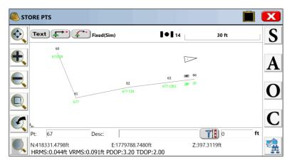
This line can be clicked within the map screen without issuing any command, and the Line Details screen will appear at left. If you tap too close to a point ID, then Point Details will appear. But you can also click lines within the command Store Points. This provides additional options to Extend the Line and draw a New Line from the nearest vertice to the picked point. These options are discussed in detail in the section on Feature Code List found in the File menu.
