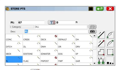
Regarding heights, the **TB** icon will toggle between the current height of measurement (e.g. prism height, antenna height) and a list of previously stored heights. It is useful when switching between commonly used heights such as full pole extension and normal setting.
