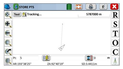
Note that in the above figure we are in "Tracking/Distance" mode for display and quick readings by S. Changing to "No Dist" mode leads to display of direction only, as shown in this figure:
