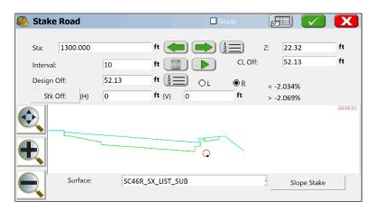
The selected or highlighted cross - section surface always appears red and bold for purposes of stakeout. The Settings button at the top of the screen leads to the standard Road Stakeout settings controls, also found in Job Settings, Stake tab.
