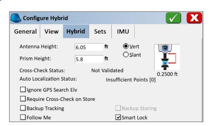
The screen shot above reflects the status of an Auto Localization routine before any points are stored. When enough points are stored the Auto Localization status will switch from 'Insufficient Points [0]'.
