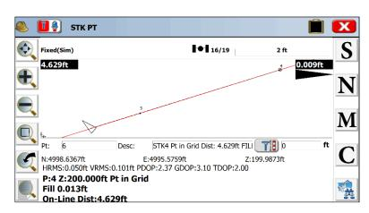
• Navigate to that line (which will turn green once within the stakeout tolerances) and store the point.
