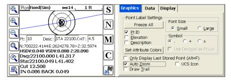
The "Story Stake" information would appear as shown below (Progressive and Total options). By staking Section ID "Ditch", there are 2 Ditch ID points to the left and 2 shoulder and 1 Center point to the right, up to the selected centerline. If "Show Report up to Center" is turned off (in effect, show ENTIRE report), then a much more complete report would appear providing offset information to all section points on both the left side and right side of the road.
