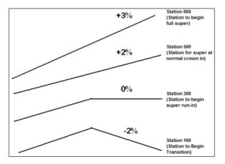
You enter all these key stations (begin, flat outside lane, reverse crown, full super) both going up to full super and transitioning back down to normal crown. Recognizing that the normal crown of -2% transitions from station 100 through a slope of 5%, the transition is 1% per 100 feet, assuming an even rate of transition. Therefore, a "flat"
