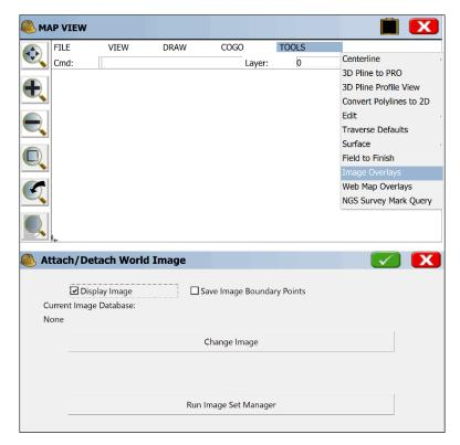
Images that do not have any georeferenced information built into them (or available in a separate jpw or tfw file) must be calibrated within Carlson X-Port, the office software companion to SurvPC, using the Image Manager. GeoPDF format is supported.
