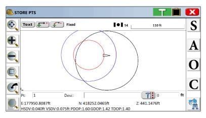
**Example 2:** The red icon in the top bar indicates that the receiver is tilted too far to correct for tilt, as configured in the tolerances dialog by the Incline Tolerance (for example, more than 20 degrees). The bubble level also shows that the receiver is very unlevel. No point can be stored.
