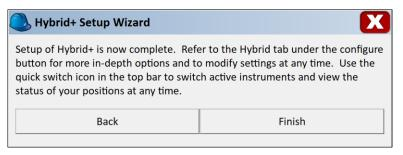
Click on 'Finish' to exit the Hybrid+ Setup Wizard. SurvCE will now automatically set the active instrument to the robotic total station. It will not be possible to switch to GPS mode until enough points are measured with the robotic total station to form a good auto localization. From the main menu, select Survey – Store Points. The Store points routine will be used to form an auto-localization.
