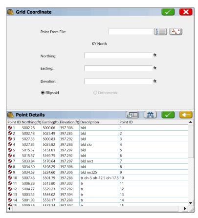
The Coordinate method is similar to the Lat/Lon method, since Lat/Longs convert to Grid Coordinates based on the current coordinate system set in Job Settings, GPS option. The Grid Coordinates will convert back to the Lat/Long coordinates needed by SurvPC to configure the base.
