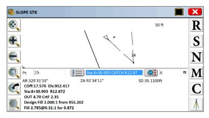
Note: When using either GPS or total stations for slope staking, you can obtain more graphics and less screen information by pressing the down - arrow key. It literally has the effect of bringing the graphic screen down (see below). Pressing the up - arrow key will pull the screen back up and show the full text. This works in all modes except GPS Simulation, where the up - arrow moves the cursor faster, down - arrow slower.
