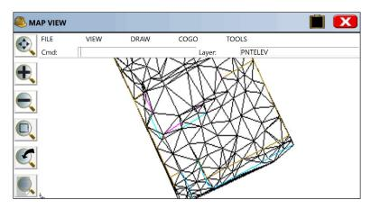
The 3DFaces are placed on a layer (TRI\_FACE by default), and that layer can be turned off and removed from view. If you choose E for Erase, you can pick the 3D Face entities and erase them on command. There is no particular value to seeing the 3D Faces, so it is not recommended that they be drawn. The main value is to capture the TIN (triangulation) file for use in Elevation Difference.
