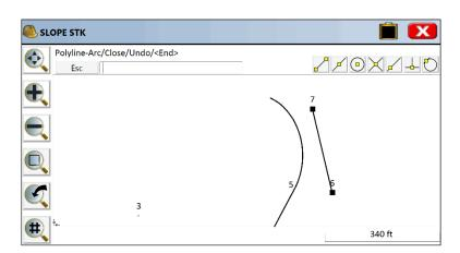
When a new horizontal alignment is selected by 3D polyline or point method, the program will ask if you wish to overwrite any existing vertical alignment selection. The typical answer is yes—you want it for both, and you are ready to stake any station at any interval based on user-entered slopes. Think of points 6 to 7 as the flow line of a ditch with steep side slopes, and the goal is to lay the slopes back at 2:1—a perfect application for Point-Defined Slope Staking.
