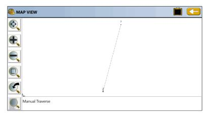
Click **Back** to return. You always have the option to enter new angle and distance information, Calculate, check the Map, then Store, as desired. **Point in Direction** offers the flexibility to check point locations graphically prior to storing.
