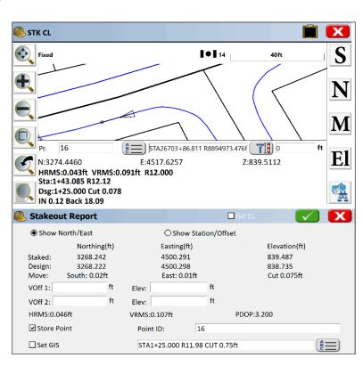
Note that you have the option to store a point in stakeout. If the point being stored is the same as one in the current job file, the **Point Protect** dialog box appears stating that the point you chose has already been used. The next available point number is listed with the option to overwrite the current point or use the new number. If you "Show Station/Offset", you will see the Station and Offset of the design (1+25.000 R12.000) and staked point (1+25.000 R11.979), for example.
