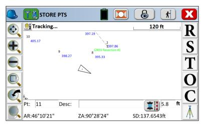
Within the Store Points screen, each time a point is stored with the robotic total station, the GPS measurement is collected at the same time. A localization will be formed in the background by analyzing all measurements pairs and selecting the best quality measurements.
