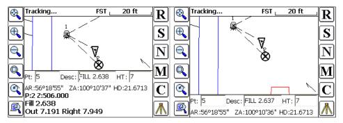
The expansion of the graphic screen in stakeout can be accomplished two ways: (1) press the down - arrow to expand, up - arrow to return to normal (at left) and (2) place your finger or stylus in the first line, near the "Desc" and pull - down and repeat the process and pull up the screen. (For restoring the full screen, the up - arrow is the easiest method).
