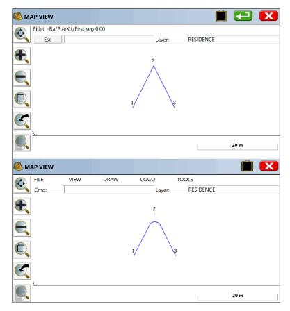
See the above two figures. Because in the Left figure, from 1 to 2 to 3 was one continuous polyline, after the radius was set at 15, P was entered to set up the one-pick approach for polylines, leading to the completed fillet command and the result as shown in the Right figure. Now you can do Cogo, Interpolate Points, Polylines to Points (P2P) and solve for the points for the beginning of the arc, radius and end of arc, for purposes of stakeout (set out).
