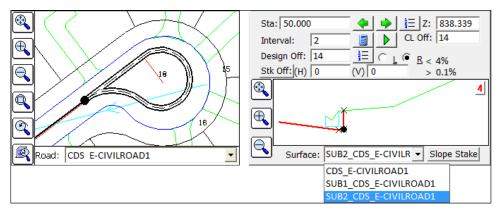
The cul-de-sac "centerline" is the outside edge-of-pavement facing the curb, and by clicking "From List" opposite Station, is seen to be just over 200 in total length in the screen below left. Staking out station 50 would be approximately 1/4 of the distance around the cul-de-sac.
