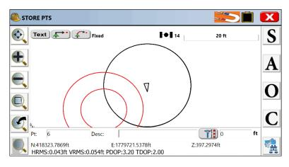
**Example 4:** To store a reading in areas of magnetic noise, simply level up the pole to within level tolerance. The icon now indicates that there is magnetic noise, but the receiver is level enough to store. Note that in this state, due to the magnetic noise, no adjustment will be made for incline.
