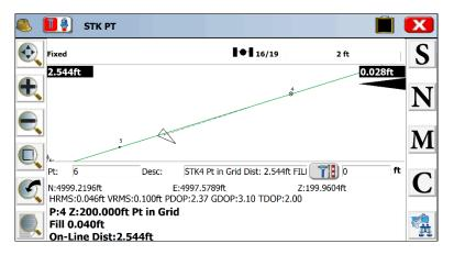
• The Obstructed Point Alignment screen will show the user the distance along that line the obstructed point can be found.
