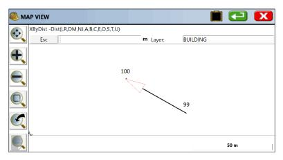
Then enter T for Total Distance (program displays current distance of 7.07), then 10 (the additional 2.93 feet is drawn), then R for Right. The arrow then turns to the right. Then enter 15 then R, then 20, R, 10, R, 10, then C to close.
