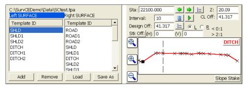
Note that when picking the first ditch point left side, that the layer is Ditch, and the next two are layered Ditch1 and Ditch2. Above the select Ditch point to the right is the third shoulder point on the left side, with SHLD2 as the ID. The next step is simply to click OK (green check) and start the normal stakeout process. Note also that you can Slope Stake (typically from the outer ditch point on the trapezoidal ditch, Ditch1 in this case).
