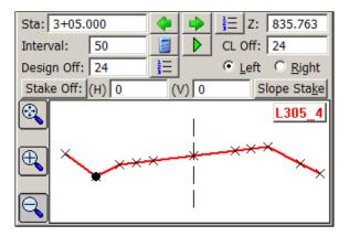
If you click Slope Stake, you can stake by the template slope for the ditch shown on the left side, or you can enter a user-defined slope to override what is in the template.
